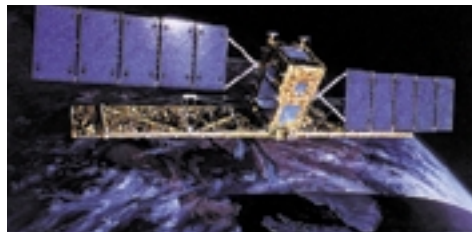
Figure 3.67 RADARSAT-1 takes pictures of Earth's surface using radar, not light.
