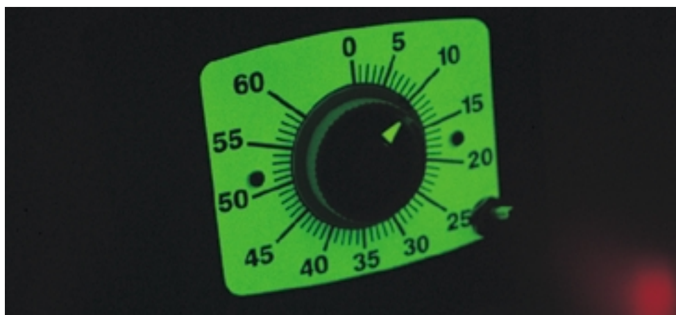
Figure 3.7 The inner surface of television and computer screens is coated with phosphors. Phosphorescent materials are also often used in photographic darkrooms. This phosphorescent dial on a darkroom timer glows to indicate how long a photograph should remain in various solutions.
