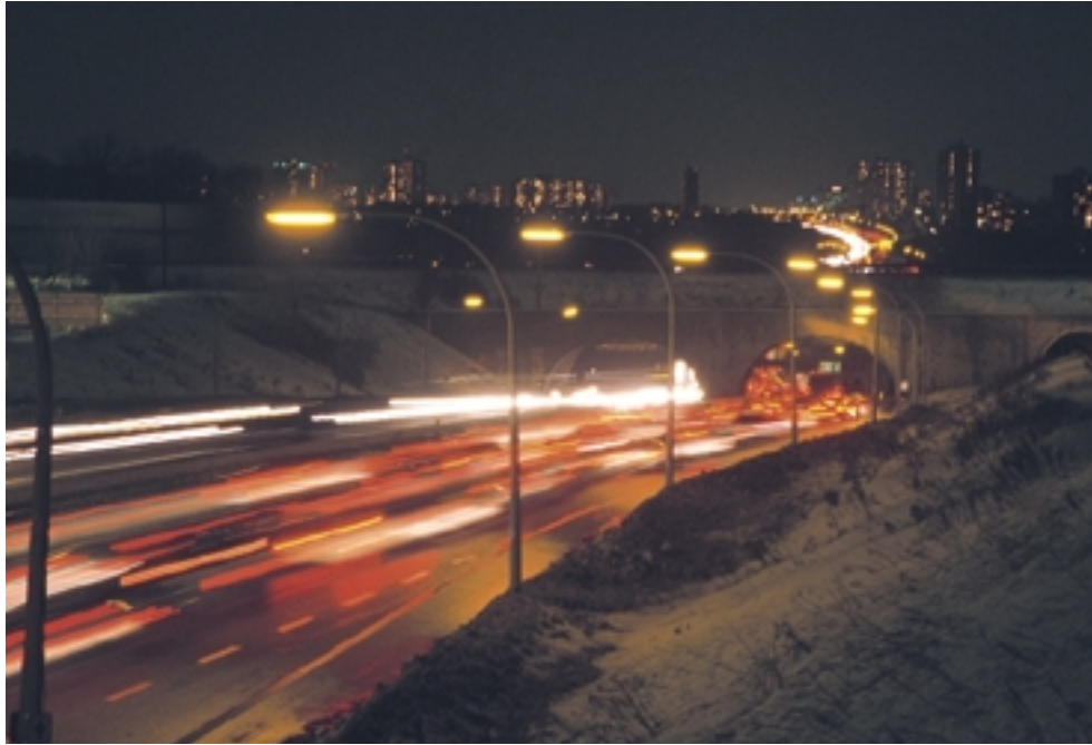
Figure 3.4 These bright yellow lights contain sodium vapour. Electricity makes the gas glow, producing a very intense yellow light.
